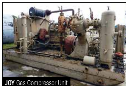
JOY Gas Compressor Unit
