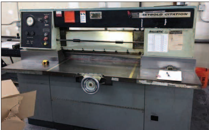
Seybold Citation Computerized Cutter Control Panel-CLB-390-D
