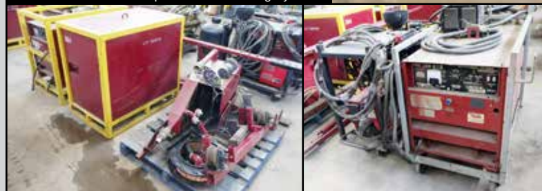
AGW 3 O'Clock Self-Propelled Girth Welding Systems
