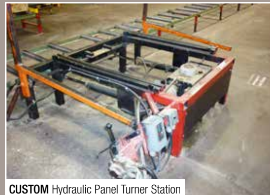
CUSTOM Hydraulic Panel Turner Station
