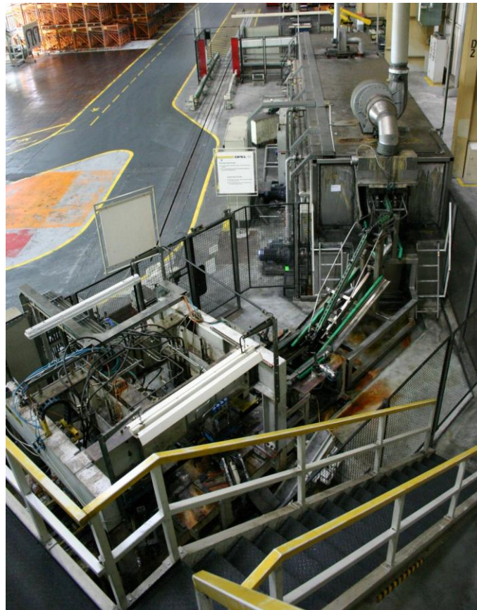
HEISS tube end machining unit loaded by FANUC robot TECHNO-COMMERZ washing/coating/drying unit
